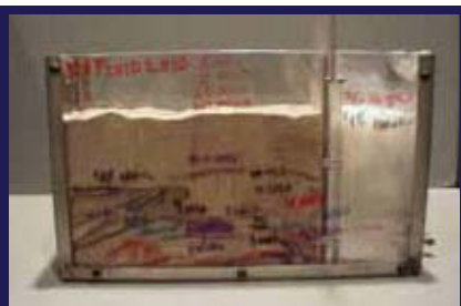
Holding Uncompacted Dry Sand Side Wall or 48 Hours
